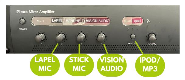
To connect an iPod/Mp3 Player connect via AUX cable into the input on the side of the unit
